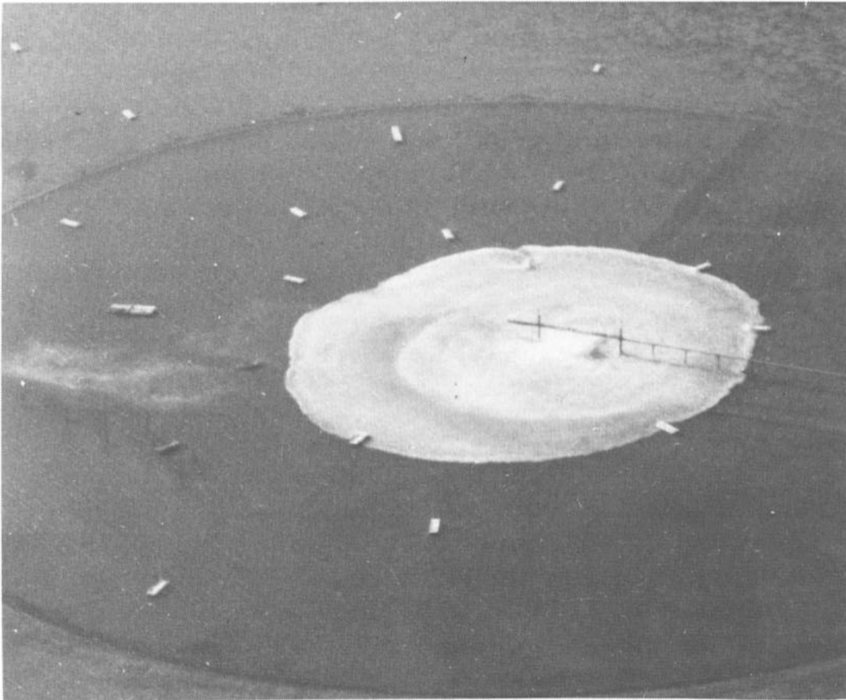
Fig. 4. Spill 60 — instantaneous propane spill of 27 \text{ m}^3 in 1.2 \text{ m/s} wind.
